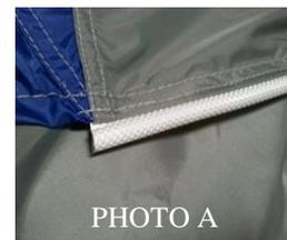
3. **Starting** at the rear of the trailer, slide the Awning keder cord into the keder rail on the passenger side of your trailer. Make sure that the Awning keder cord is able to feed freely into the rail as you pull the Awning towards the front of the trailer. The Awning keder cord should fit completely into the rail, with little or no excess hanging out on either end.
